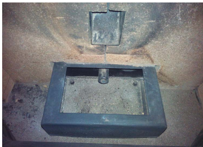
Figure 35: Remove ash from ignitor tube (underneath repot)
