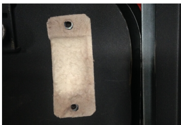
Figure 36: Remove lower exhaust chamber's cover plate and clean
